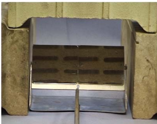
Fig. A3.2 Camcorder view of the swivelling mirror of Prototype 1 inspection system at a cold test checker brick
