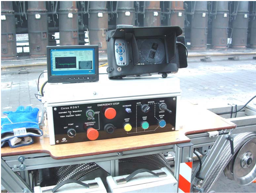
Fig. A6.16 Control system and data display with head temperature graph (on the left) and flue video (on the right)
