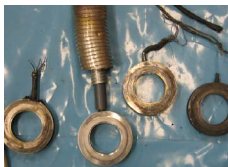
Fig. A3.16 Three damaged cables and load washers and improved one in centre
