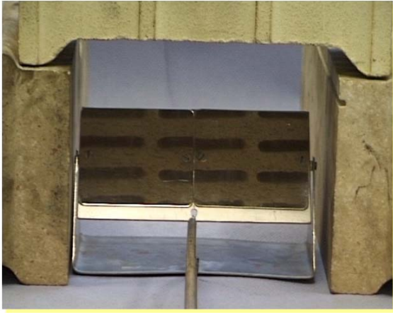
Fig. 15 Camcorder view of the swivelling mirror of Prototype 1 inspection system at a cold test checker brick
