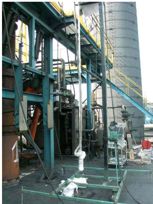
Fig. A1.6 Camera head fixed at the end of a tube before introduction inside an empty oven
