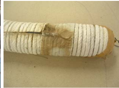
Fig. A3.11 After test, insulation shows no adverse effects
