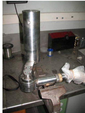
Fig. A2.2 Camera head without insulation
