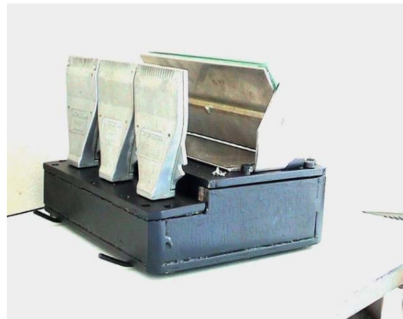
Fig. 17 Combined inspection/cleaning system
