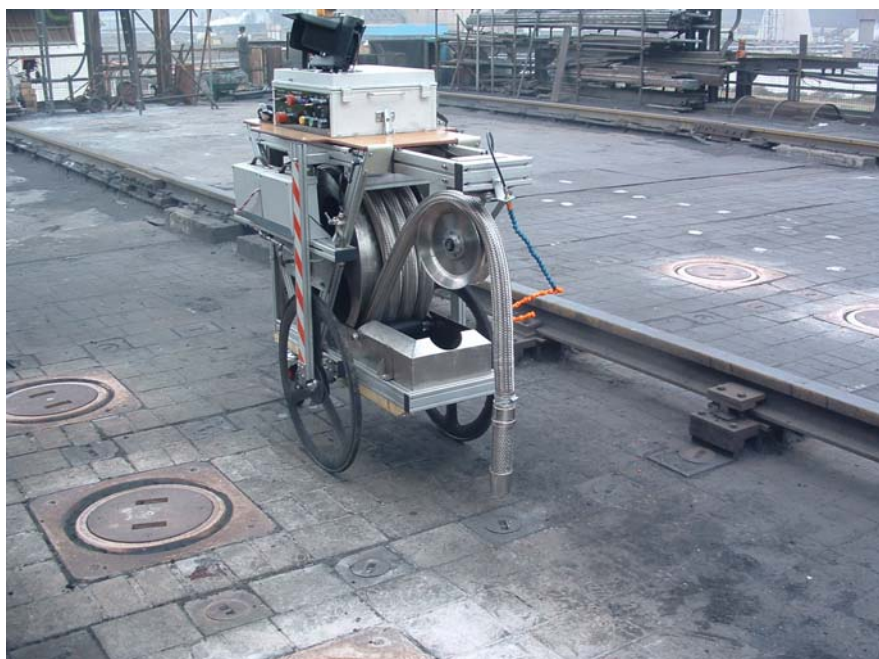
Fig. 32 Automated flue temperature and vision monitor in position on the battery top
