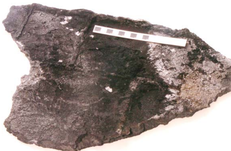
Fig. A2.7 Wall carbon deposits - L: brick pattern from wall, N: globular laminar carbon on coke-side
