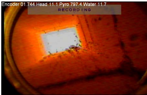
Fig. A6.20 Wall 44, Flues 6 (on the left) and 7 (on the right) 1.7 m from the battery top
