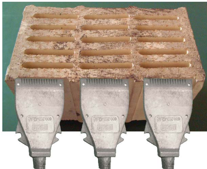
Fig. 1.16 Parallel connection of 3 selected nozzles adapted to the length of checker brick slots
