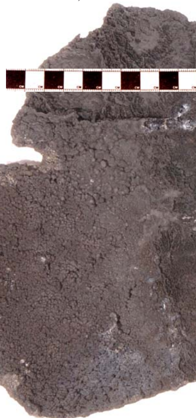
Fig. A2.7 Wall carbon deposits - L: brick pattern from wall, N: globular laminar carbon on coke-side
