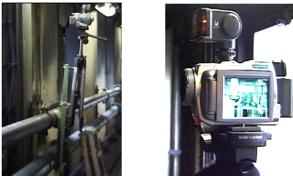
Fig. A3.6 New camcorder with additional illumination
