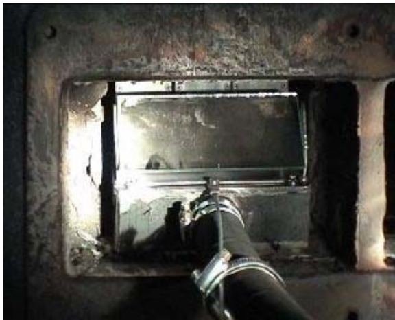
Fig. A6.22 Insertion of the Prototype 2 inspection/cleaning system into the sole flue
