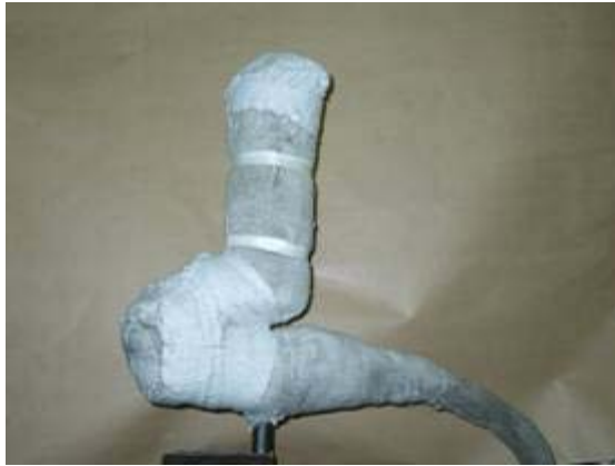
Fig. A1.4 Insulated camera head
