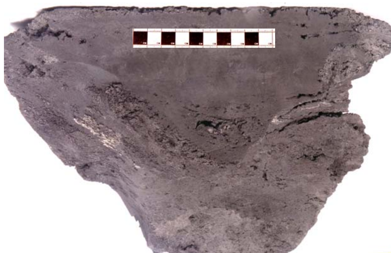
Fig. A2.6 Layering in Sample A roof carbon deposit parallel to the oven wall
