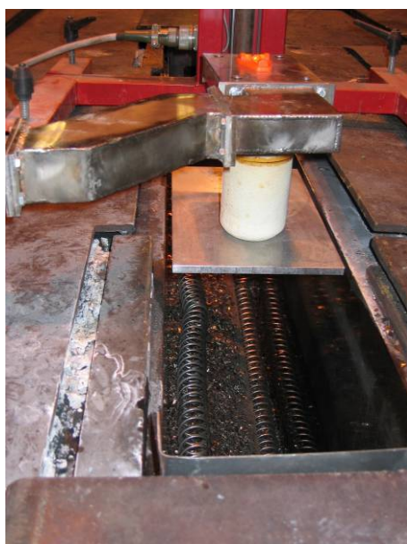
Fig. 39: Calibration of the level sensor used together with the meniscus velocity sensor in the mould (MEFOS)
