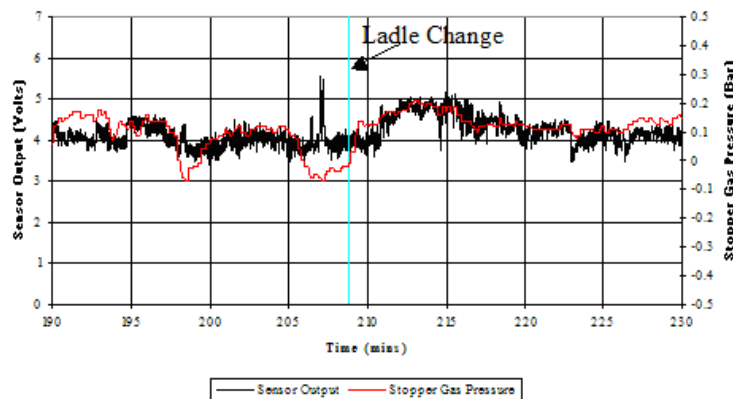
Fig. 73: Output from sensor and stopper gas pressure during trial 13 (Corus)
