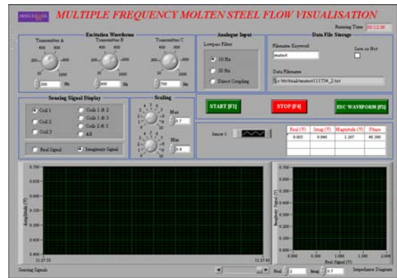
Fig. 1b: New multi-frequency electromagnetic SFV sensor user interface screen (Corus)
