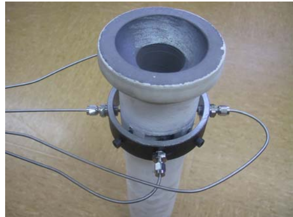
Fig. 14: New fixing method to guarantee a good contact between the thermocouples and the refractory nozzle body (Sidenor)
