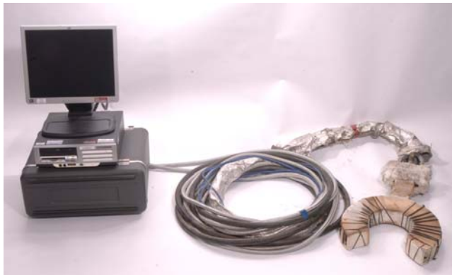
Fig. 1a: New multi-frequency electromagnetic steel flow visualisation sensor (Corus)
