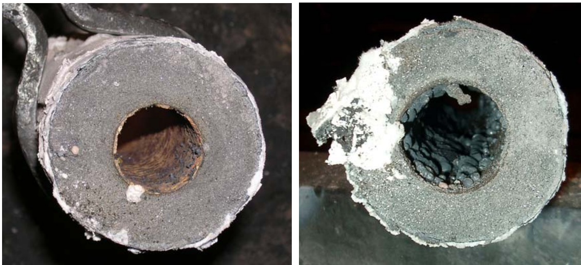
Fig. 62: Clogging observed at the SEN: left: no clogging after casting of sequence no 7, right: light clogging after casting a sequence at which no measurement results could be received (BFI)
