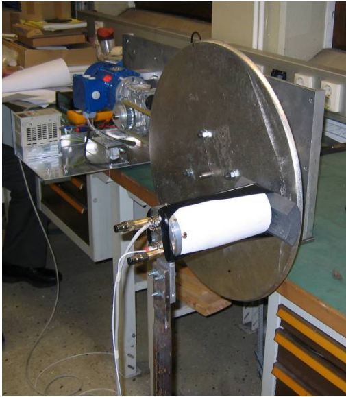
Fig. 31: Calibration of SEN flow sensor in the calibration rig (MEFOS)
