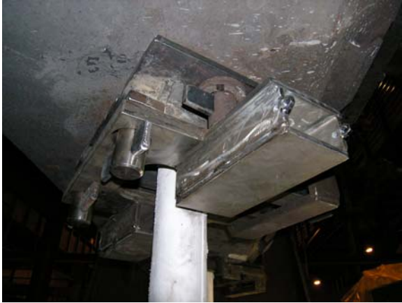
Fig. 7a: Sensor holder before tundish preheating (Saarstahl)
