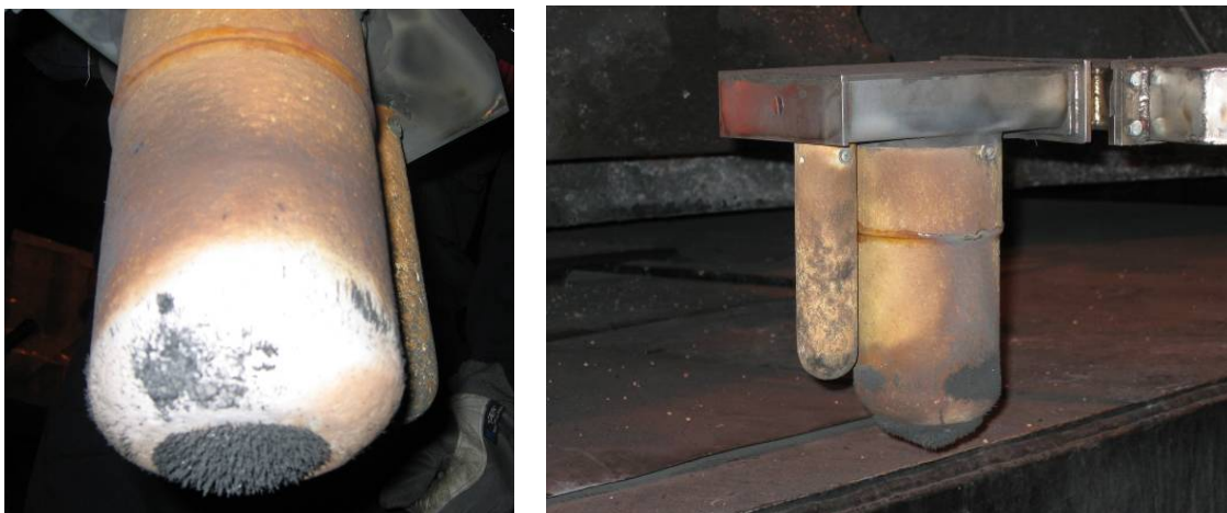
Figs. 41a and 41b: Casting powder on the house of the meniscus velocity sensor (MEFOS)
