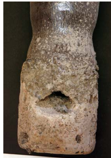
Fig. 94: SEN from trial 17 with 71% reduction in exit port size (Corus)
