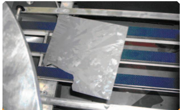
Broken wafer during thin wafer test run
