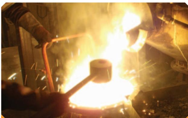
H29 furnace for upgraded metallurgical-grade Si
