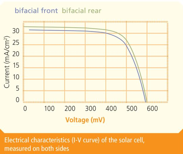
Electrical characteristics (I-V curve) of the solar cell, measured on both sides
