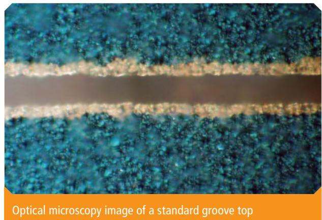
Optical microscopy image of a standard groove top
